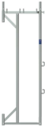
VERTICAL FRAME FOR ROOF OVERHANGS Steel tube Ø 48.3 mm, hot dip galvanized, for retrofitting roof overhangs. PU: 25 pieces
