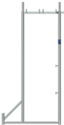
CONVERSION FRAME Steel tube Ø 48.3 mm, hot dip galvanized, for converting a 3-board frame into a 2-board frame. PU: 25 pieces
